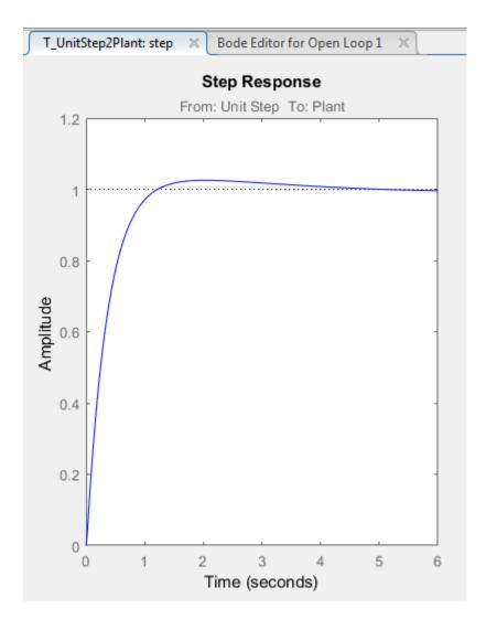
The plot shows that the closed-loop response of the system is stable. The system with the designed controller thus meets both the magnitude and phase margin requirements.
