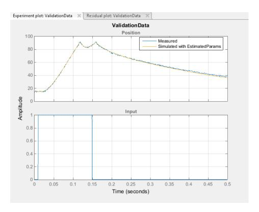
The simulated response as shown in light brown on the top experiment plot is overlaid on the measured out put data, and closely matches the measured validation data.
