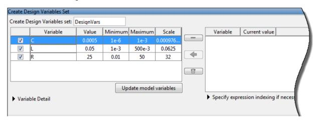
A new variable <code>DesignVars</code> is created, and appears in the <code>Data</code> area of the Response Optimization tool.
