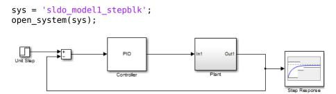
The model includes a Step Response block which is a Check Step Response Characteristics block from the Simulink Design Optimization **Model Verification** library and has default step response bounds.
