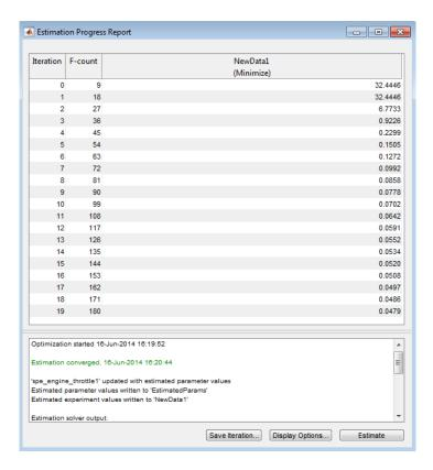
The estimated parameters are saved in the Parameter Estimation tool, in the **Results** section of the **Data Browser** pane, as <code>EstimatedParams</code>. Right-click <code>EstimatedParams</code>, and select **Open...** to view the results.
