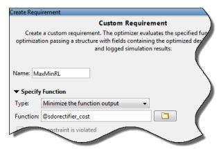
A new requirement variable MaxMinRL is created, and appears in the **Data** area in the Response Optimization tool. The **Iteration plot 1** tab shows the value of MaxMinRL at each iteration during the optimization.
