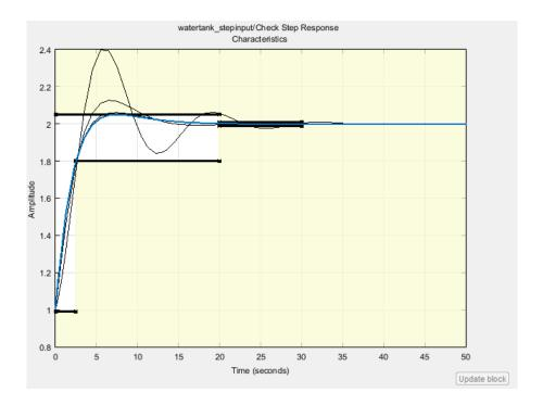
The plot displays the last five iterations. The final response using the optimized variable parameter appears as the thick blue line. The optimized response lies in the white region bounded by the design requirement line segments and thus meets the requirements.
