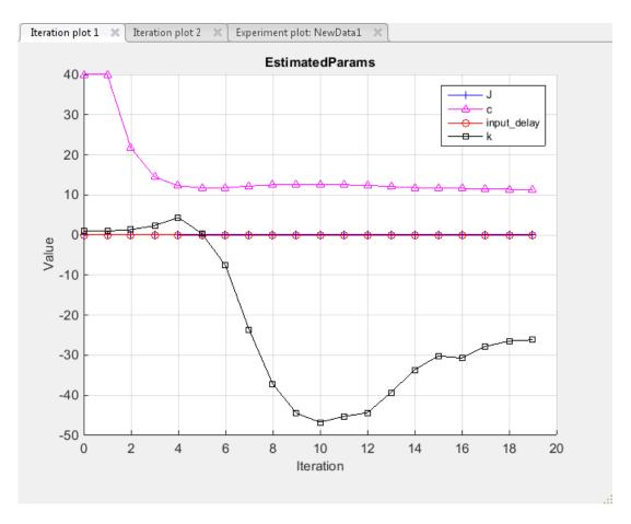
The **Estimation Progress Report** shows the iteration number, number of times the objective function is evaluated, and the value of the cost function at the end of each iteration. After the estimation converges, the **Estimation Progress Report** looks like this figure.
