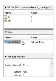
If your model has many parameters, you can first use sensitivity analysis to determine the most influential parameters to optimize, or to obtain initial guesses for the design variables. To open the **Sensitivity Analysis tool**, in the **Response Optimization** tab,
