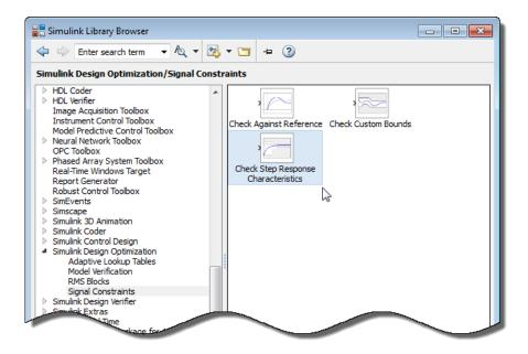
Drag and drop the Check Step Response Characteristics block into the model window and connect the block to the output. The block is connected to the signal for which you want to specify design requirements.
