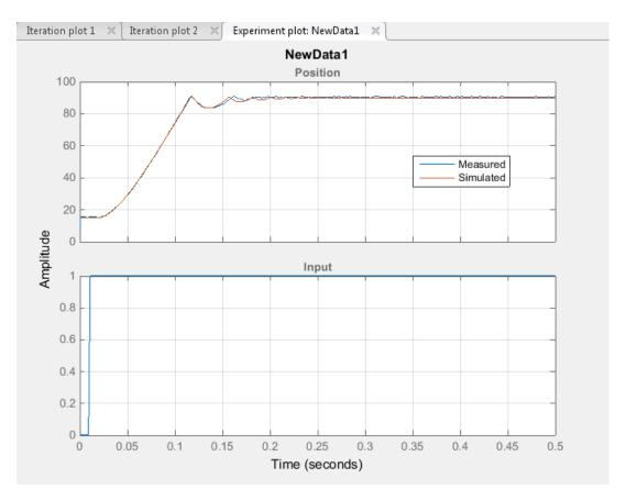
The data simulated using the estimated parameter values agree better with the measured data than when the parameter limits were not specified.
