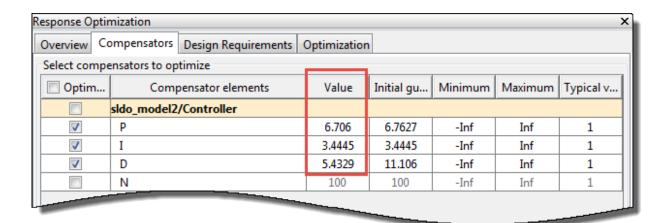
**6** Write the optimized controller parameter values to the Controller block in the Simulink model.
