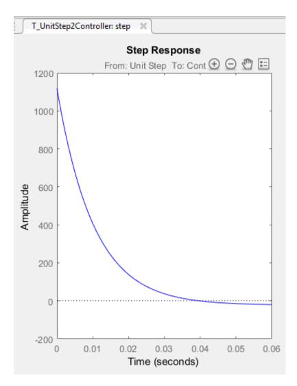
The plot shows that the peak value of the controller output is about 1100, which is large and can damage the plant. To limit the controller output, apply lower and upper bounds on the signal, as specified in "Design Requirements" on page 4-5.
