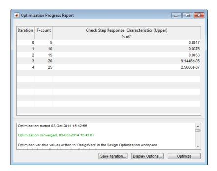
The message Optimization converged in the Optimization Progress Report indicates that the optimization solver found a solution that meets the design requirements within the tolerances and parameter bounds. For more information about the outputs displayed in the optimization, see "Iterative Display" (Optimization Toolbox).
