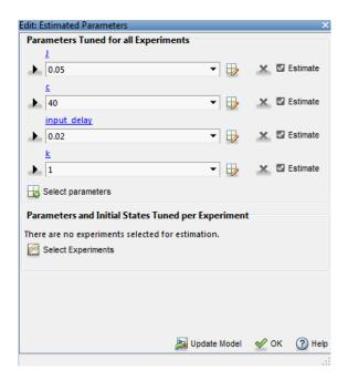
The tool selects the parameters you add for estimation by default. When estimating a large number of parameters, you can first select a subset of parameters to estimate.
