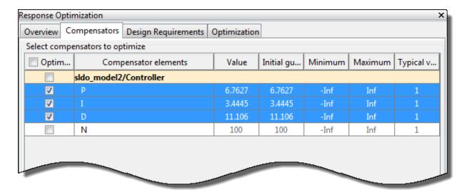
b In the **Optimization** tab, click **Start Optimization**. At every optimization iteration, the optimization method reduces the distance between the current response and the upper and lower bounds on the signal. After the optimization completes, the **Optimization** tab displays the optimization iterations and status.
